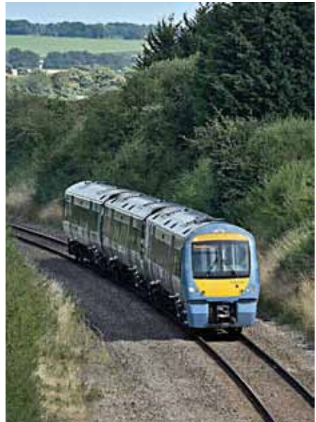
A Class170 at Wilbraham in 2014, clearly showing original position of second track, removed by BR in 1980s. CB.
