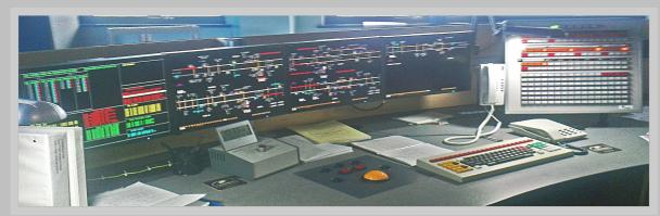
crossings at, for example, Ely station. The signaller operates the line solely from the computer screens, which have failed on two occasions and needed to be rebooted, during which time all trains are brought to a halt as the signals all go red.
