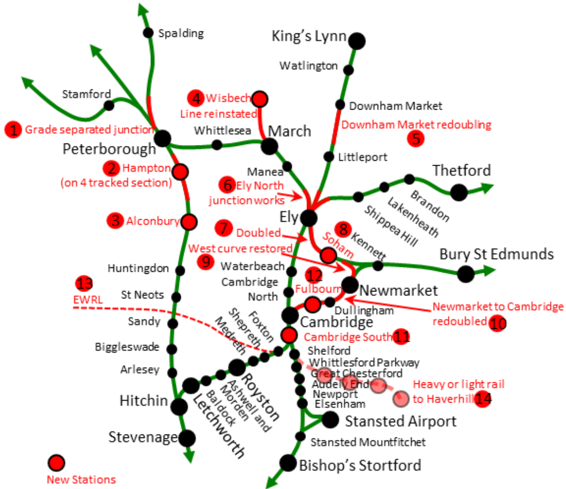
Map showing 14 key upgrades which are required on the railway network in Cambridgeshire and Peterborough
