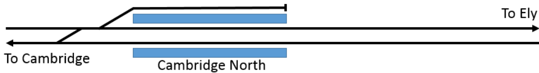
1. Track layout of Cambridge North as proposed by Network Rail. Limited capacity for future expansion.
