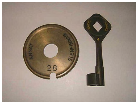
Examples of single line tokens: Tablet on left, key token on right
