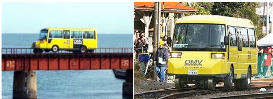
Figure 70 - shows the dual mode vehicle runs along the tracks of the Gakunan Railway Line during a trial run in Fuji, Shizuoka Prefecture.
