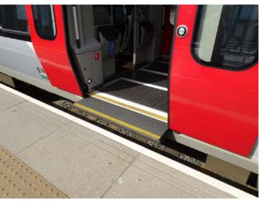
Extended step and tip-up seats on a FLIRT
