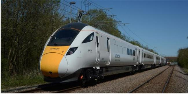
Hitachi's DfT-specified class 800 series 140mph-capable, HS1-compatible electric or electric / diesel bi-mode.
