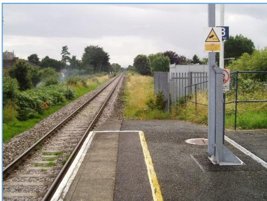
*Photo 3. West from Whimble station. The existing former down line could become the through line and the old up line restored for trains stopping at the station.*
