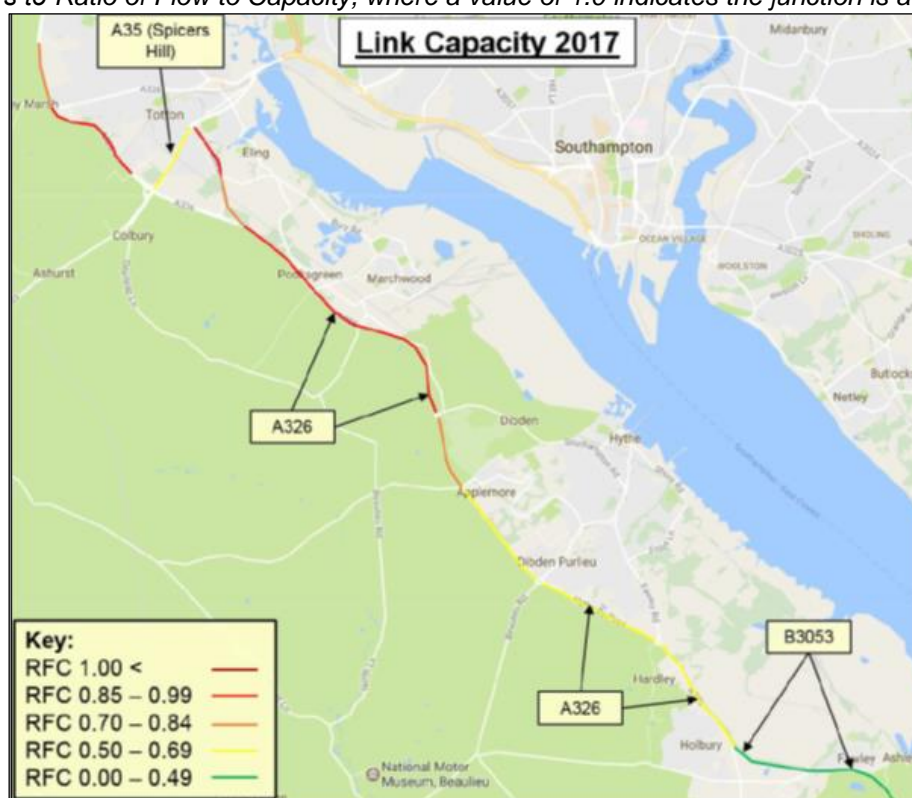
Figure 3-6- Map showing sections where A326 is operating above or near capacity in 2017 (‘RFC’ refers to Ratio of Flow to Capacity, where a value of 1.0 indicates the junction is at capacity)
