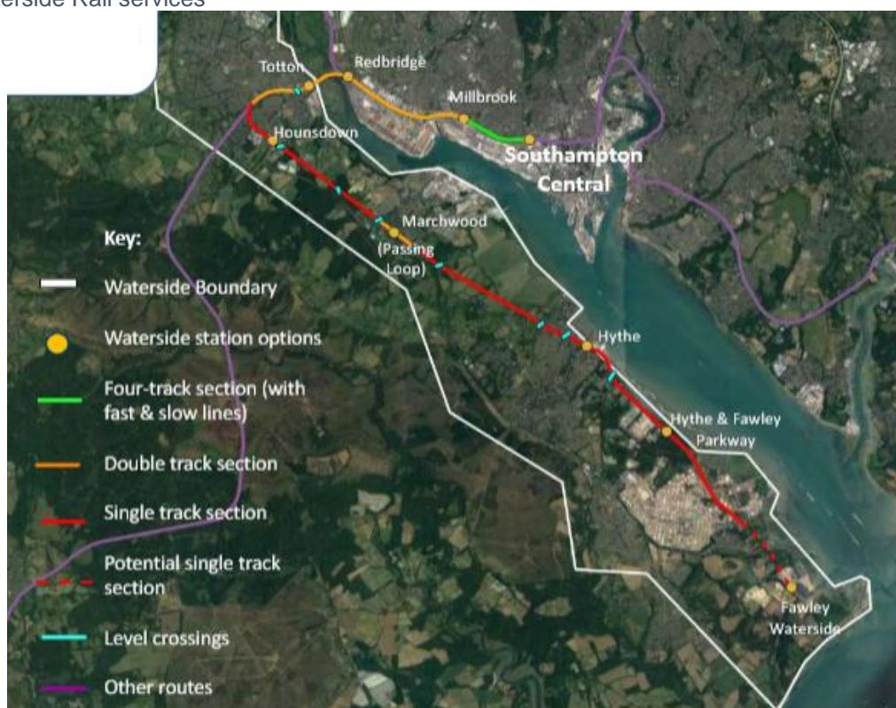
Figure 3-14 – Long List of Locations of existing and proposed stations that have been considered for Waterside Rail services
