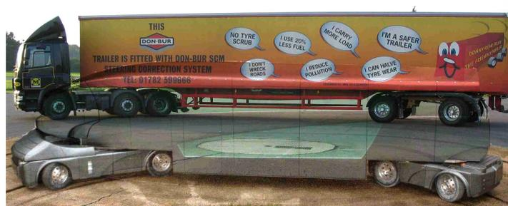
So, how does this invention help rail campaigners? Put simply, existing road-rail vehicles, which are tend to be vegetation clearance and track maintenance, are quite short. The BladeRunner bogies can be coupled to any body configuration allowing lorries and coaches to run on railway lines as long as there is a flat surface on which vehicles and join and leave the track.
