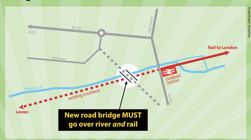
Stage one: Uckfield's planned road must make room for the railway to pass beneath
