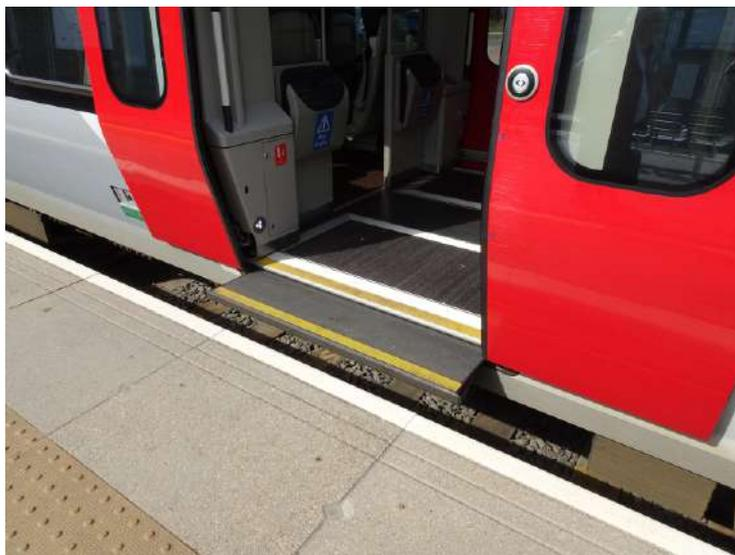
*Extended step and tip-up seats on a FLIRT*
